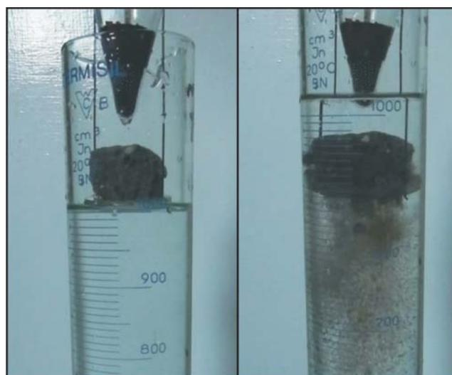
Fig. 12. Soaking of a grey-brown brick: left photograph – sample prior to inserting in water, right photograph – desintegration of a sample after inserting in water.
