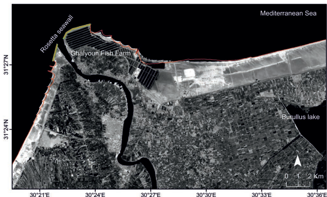
Fig. 13. Projected shoreline position in 2030 (red line), assuming no further coastal changes.
