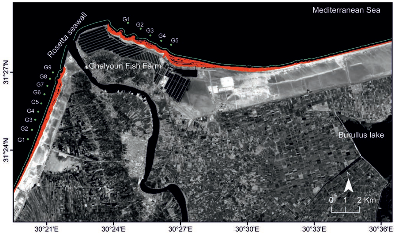
Fig. 9. DSAS input data: offshore baseline (dark green line) and 20 extracted shorelines (red lines) for the period 1999–2019.
